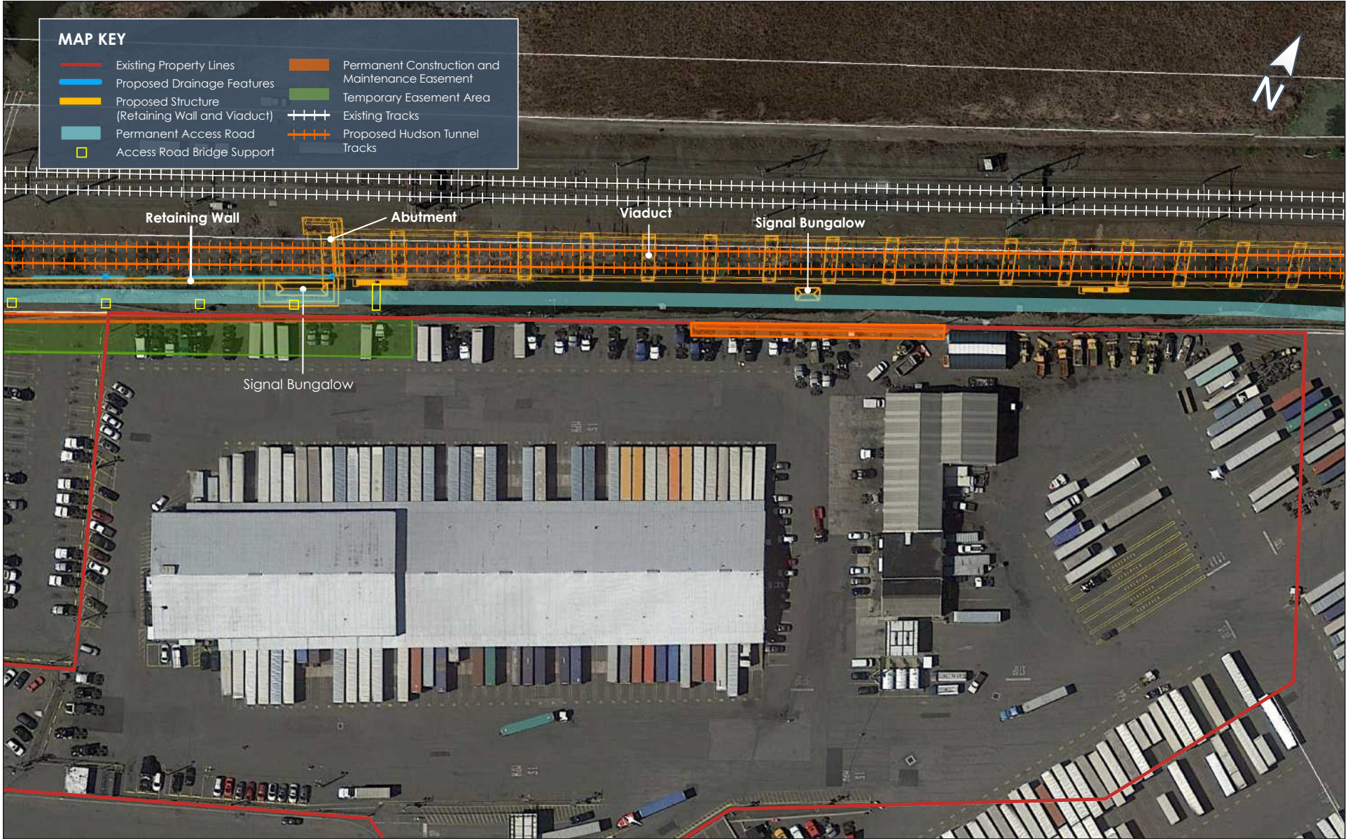
Construction Activity and Property Acquisition at 2820 16th Street, North Bergen
